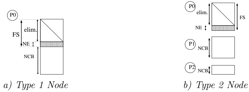
Figure 2.3: Example of mapping of the L factors of a frontal matrix. FS , elim , NE , NCB hold respectively the fully summed, eliminated, non-eliminated and contribution variables
