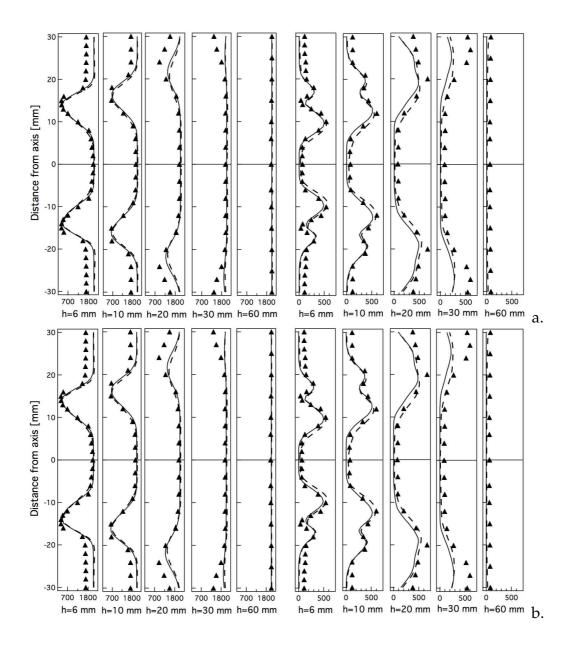
Fig. 10. a. Mean and b. RMS temperature profiles for the 'quiet' flame ( $\phi = 0.83$ ) at five sections in the chamber. The experimental results (symbols) are compared to numerical data: perfect premixed (case C - solid line) and non perfect premixed simulation (case D - dashed line).
