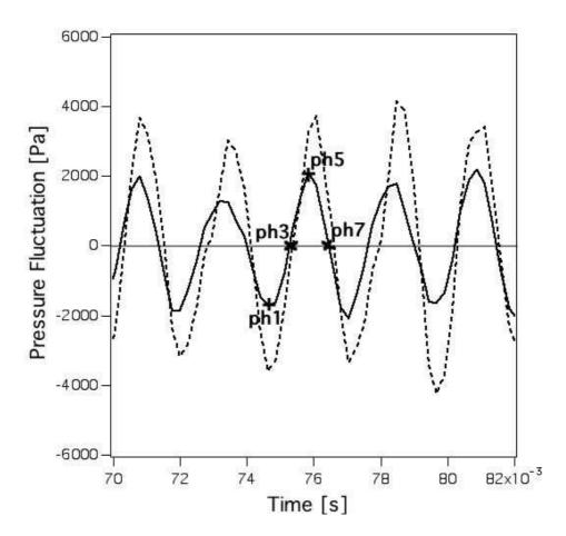
Fig. 20. Temporal evolution of the plenum pressure  $P_P$  at probe P in Fig. 1 (solid line) and the pressure drop  $\Delta P$  (dashed line) between plenum and chamber (probe C in Fig. 1) for the 'pulsating' flame (case D).
