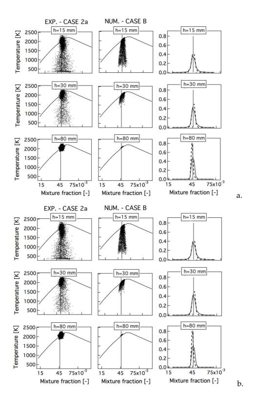
Fig. 9. a. Experimental (case 2a) and numerical (case B) correlation between temperature and mixture fraction for the 'quiet' flame ( $\phi = 0.83$ ) at h = 15,30 and 80 mm. b. Experimental (case 2a - solid line) and numerical (case B - dashed line) distribution of the mixture fraction at h = 15,30 and 80 mm for the 'quiet' flame.
