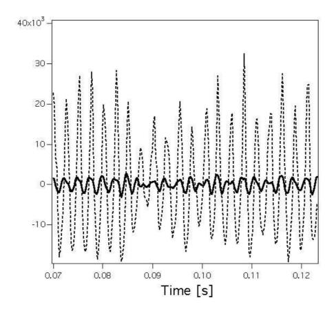
Fig. 19. Temporal evolution of the fluctuations of chamber pressure  $p_C$  (solid line, probe C in Fig. 1) and total heat release q (dashed line) for the 'pulsating' flame (case D).
