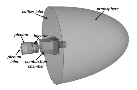
Fig. 5. Schematic of the computational domain.
