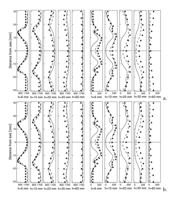
Fig. 17. a. Mean and b. RMS temperature profiles for the 'pulsating' flame ( $\phi$  = 0.7) at five sections in the chamber. The experimental results (symbols) are compared to numerical data: perfect premixed (case C - solid line) and non perfect premixed simulation (case D - dashed line).
