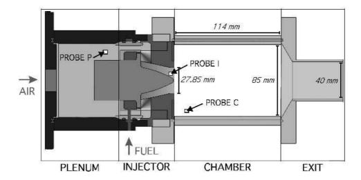
Fig. 1. Schematic of the experimental burner design [9–11]. Probe P is located in the plenum at h = -70 mm. Probe I is located in the injector before the swirler exit (h = -5 mm) and probe C is in the chamber at h = 10 mm.
