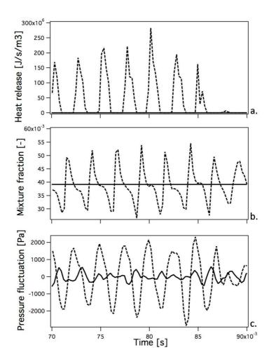
Fig. 13. Temporal evolution of the heat release (a.), mixture fraction (b.) and pressure (c.) at probe I for the 'pulsating' flame ( $\phi = 0.7$ ). Comparison between perfectly premixed simulation (case C - solid line) and non perfectly premixed simulation (case D - dashed line).
