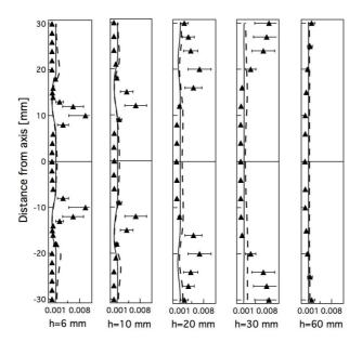
Fig. 12. Mean CO species profiles for the 'quiet' flame ( $\phi = 0.83$ ) at five sections in the chamber. The experimental results (symbols) are compared to numerical results: perfectly premixed simulation (case A - solid line) and non perfectly premixed simulation (case B - dashed line).
