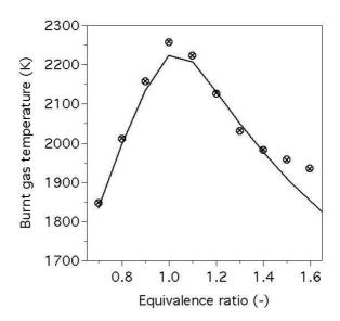
Fig. 4. Burnt gas temperature versus equivalence ratio. Comparison between GRI3.0 mechanism (——), equilibrium results (×) and 2S\_CH4\_BFER scheme ( $\circ$ ) at pressure P=1 atm and fresh gas temperature  $T_f=300$  K.
