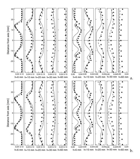
Fig. 18. a. Mean and b. RMS  $CO_2$  profiles for the 'pulsating' flame ( $\phi = 0.7$ ) at five sections in the chamber. The experimental results (symbols) are compared to numerical data: perfect premixed (case C - solid line) and non perfect premixed simulation (case D - dashed line).
