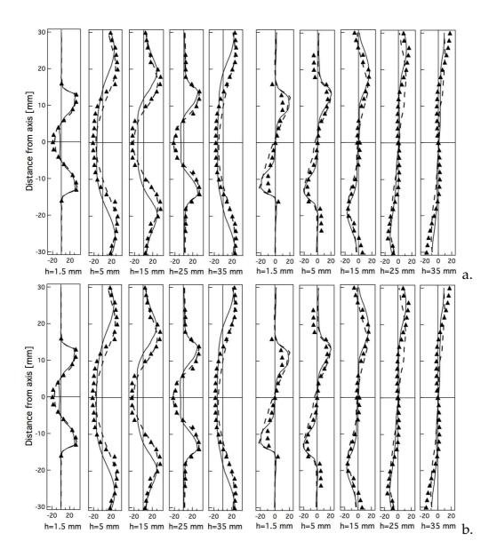
Fig. 16. Mean a. axial and b. radial velocity profiles for the 'pulsating' flame ( $\phi = 0.7$ ) at five sections in the chamber. The experimental results (symbols) are compared to numerical results: perfectly premixed simulation (case C - solid line) and non perfectly premixed simulation (case D - dashed line).
