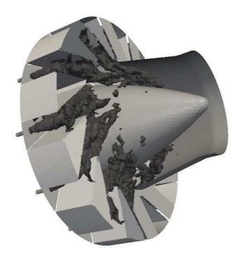
Fig. 7. Detail of the twelve computational holes upstream of the swirler for the methane injection (LES's numerical cases B and D in Table 2). Instantaneous isosurface of methane mass fraction equal to 0.5.
