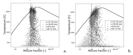
Fig. 2. Correlation between temperature and mixture fraction at section  $h=6\,mm$  for a., the 'quiet' flame (case 2a in Table 1) and b., the 'pulsating' flame (case1). Symbols represent single-shot Raman measurements at different radial positions. The solid line shows the equilibrium temperature whereas the vertical dashed line indicates the global mixture fraction (experimental data from [11]).
