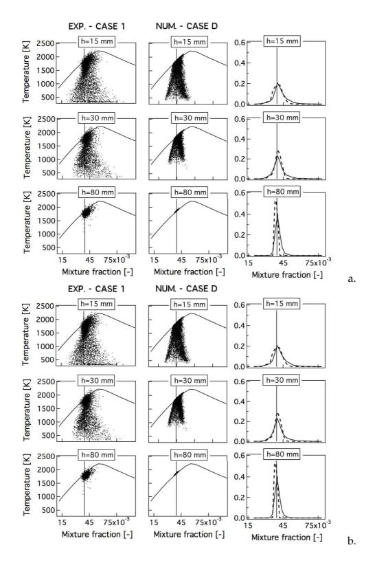
Fig. 15. a. Experimental (case 1) and numerical (case D) correlation between temperature and mixture fraction for the 'pulsating' flame ( $\phi = 0.7$ ) at h = 15,30 and 80 mm. b. Experimental (case 1 - solid line) and numerical (case D - dashed line) distribution of mixture fraction at h = 15,30 and 80 mm for the 'pulsating' flame.
