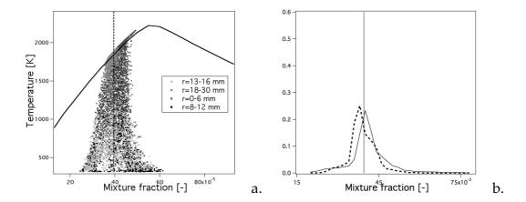
Fig. 14. a. Numerical correlation between temperature and mixture fraction for the 'pulsating' flame ( $\phi = 0.7$ ) at h = 6 mm (case D). b. Experimental (case 1 - solid line) and numerical (case D - dashed line) distribution of mixture fraction at h = 6 mm for the 'pulsating' flame ( $\phi = 0.7$ ). The global mixture fraction is indicated by the vertical line.
