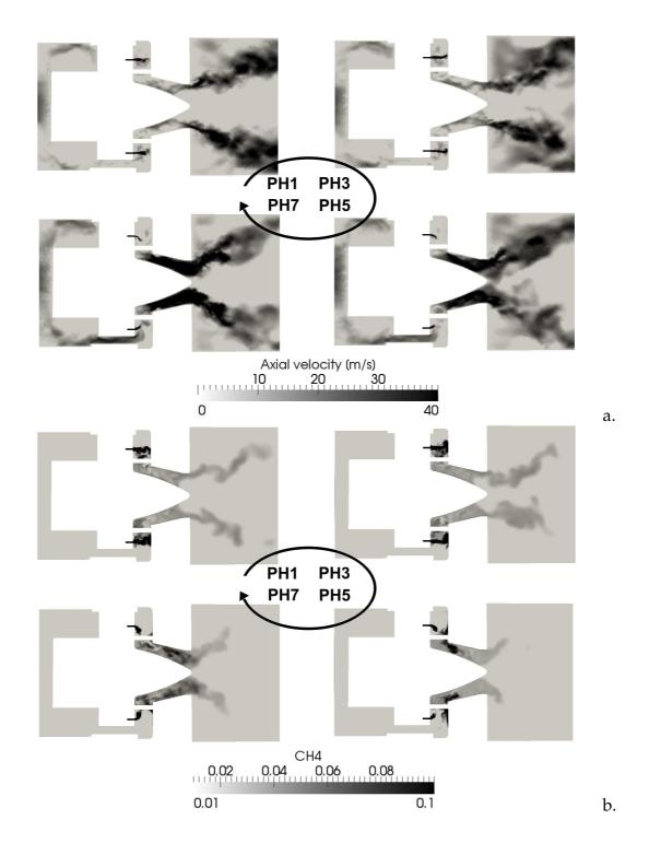
Fig. 21. Phase-locked instantaneous fields of a. axial velocity and b.  $CH_4$  mass fraction for four different phases ph1, ph2, ph3 and ph4 for the 'pulsating' flame ( $\phi = 0.7$ , case D).
