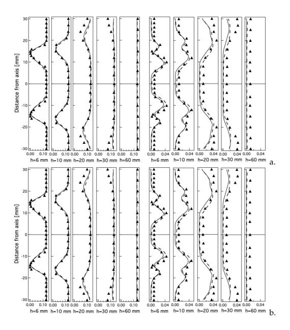
Fig. 11. a. Mean and b. RMS  $CO_2$  profiles for the 'quiet' flame ( $\phi = 0.83$ ) at five sections in the chamber. The experimental results (symbols) are compared to numerical data: perfect premixed (case C - solid line) and non perfect premixed simulation (case D - dashed line).
