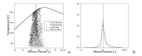
Fig. 8. a. Numerical correlation between temperature and mixture fraction for the 'quiet' flame ( $\phi = 0.83$ ) at h = 6 mm (case B). b. Experimental (case 2a - solid line) and numerical (case B - dashed line) mixture fraction distribution at h = 6 mm for the 'quiet' flame ( $\phi = 0.83$ ). The global mixture fraction is indicated by the vertical line.
