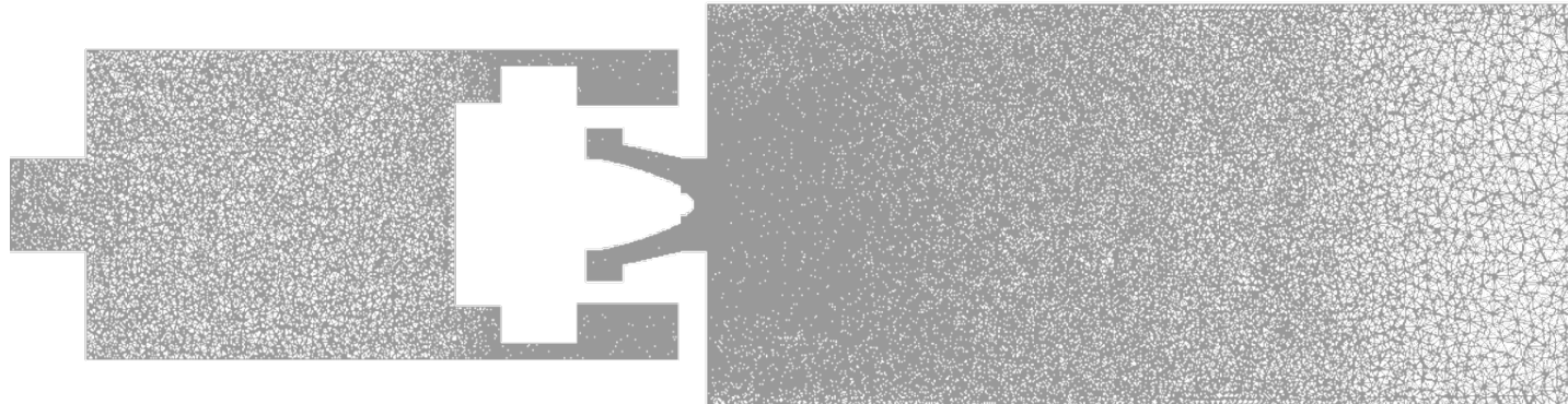
Mesh in the median cut plane (2 000 000 nodes)
