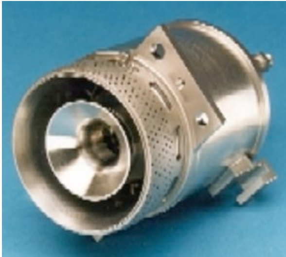
LP injection system (RR)
