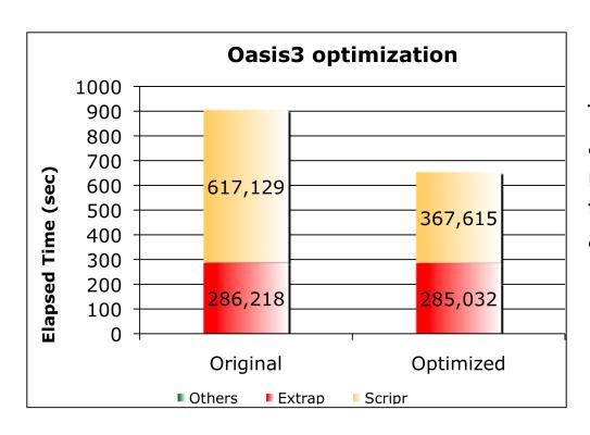
The optimization of the *extrap* and *scripr* routines gets a reduction of elapsed time on the whole coupling operation of about 27%
