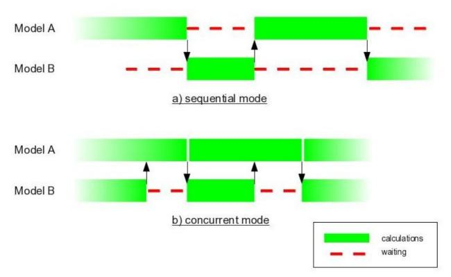
Fig 1 : Sequential, concurrent mode, on a coupled system including 2 models
