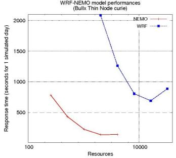
Figure 5 : Model scalabilities of WRF and NEMO model as part of a coupled system
