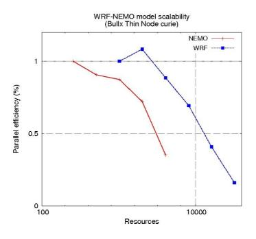
Figure 6: WRF and NEMO model parallel efficiency on coupled mode
