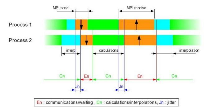
Figure 2 : En, Cn et Jn (jitter) definition, during send/receive operations, for 2 processes of an MPI parallel model (n)
